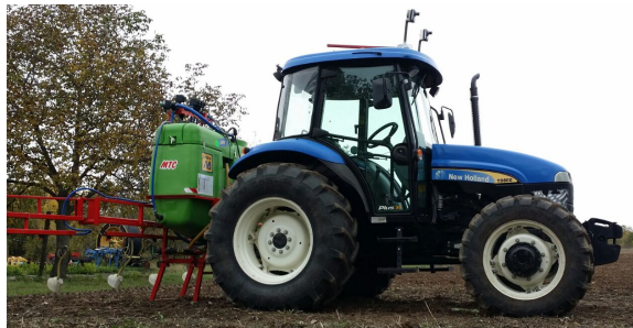
Fig. 1. Experimental model of the smart system for active control of work for performing phytosanitary treatments
